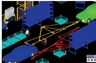
3D view of 2-operator assembly line workplace animation involving moving products.
